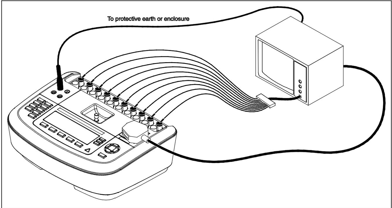
**Figure 4. DUT Connections to the Analyzer**
