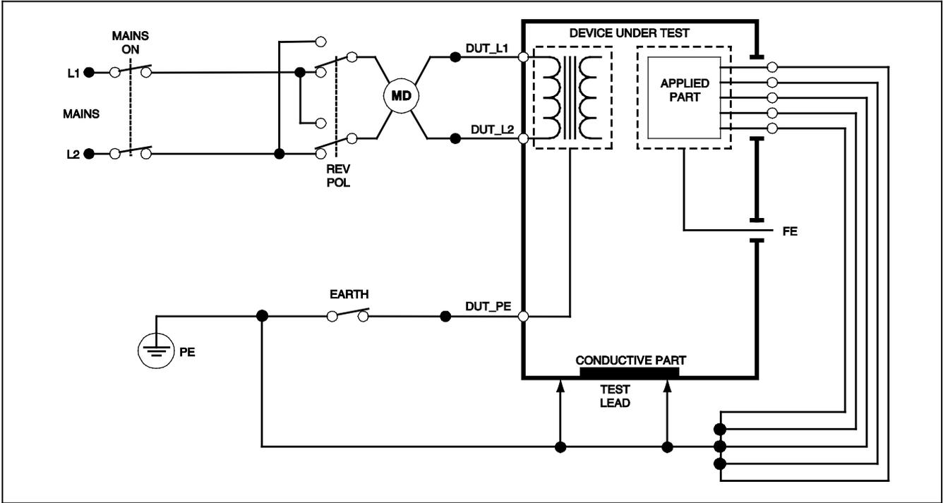
**Figure 29. Differential Leakage Current Test Schematic**
