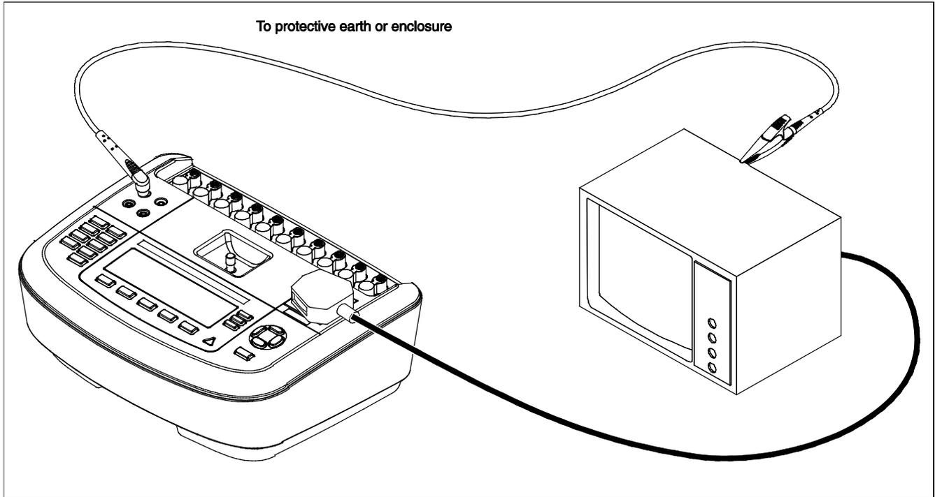
**Figure 7. 2-Wire Earth Resistance Measurement Connections**
