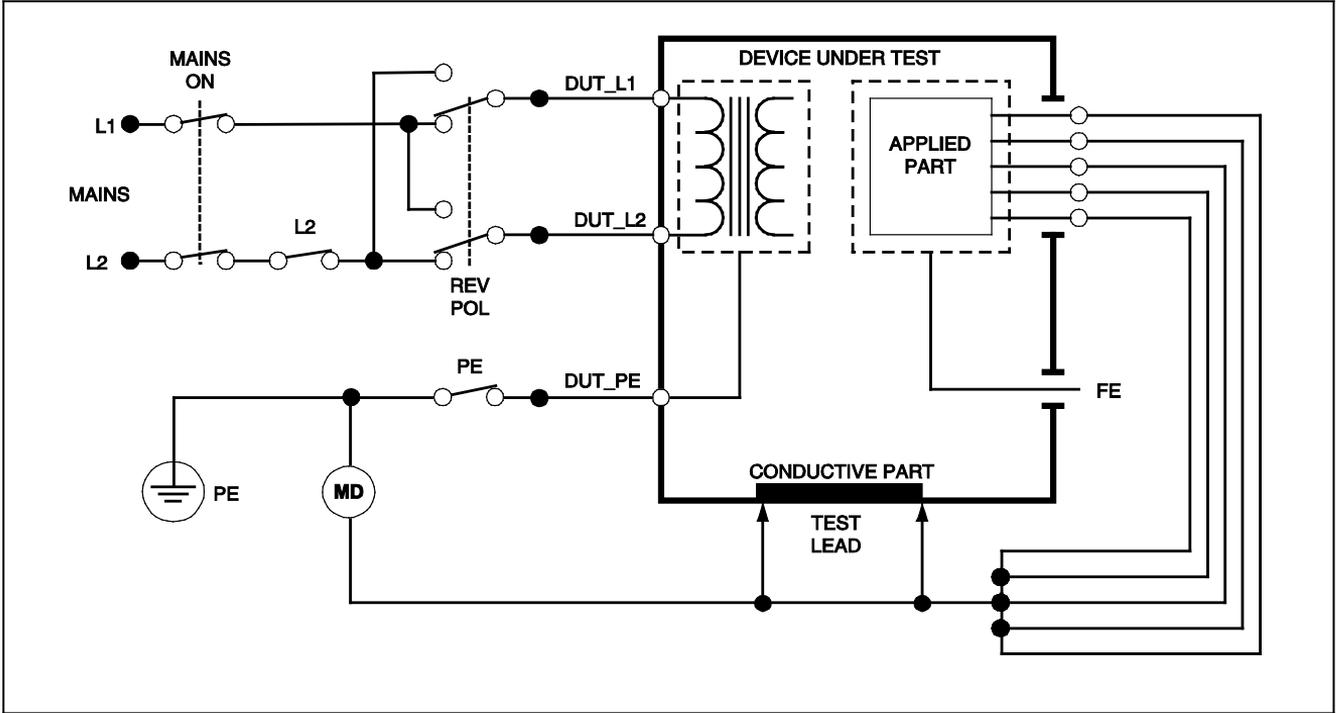
Figure 27. Direct Equipment Leakage Test Schematic
