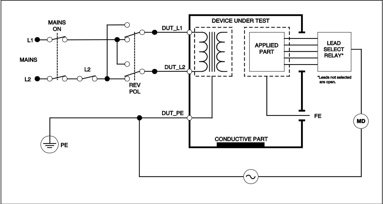
Figure 28. Direct Applied Parts Leakage Current Test Schematic
